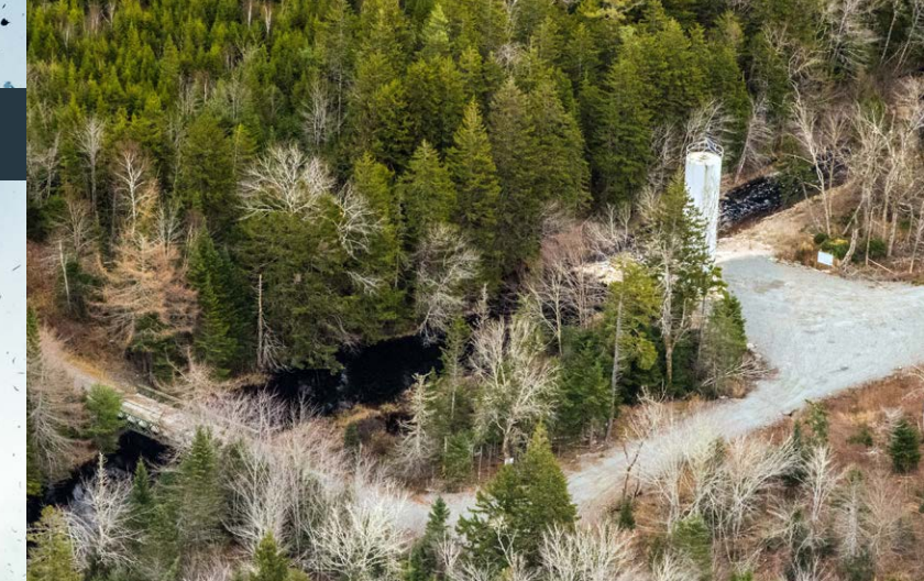
A lime dozer that the NSSA set up on the Killag River to restore wild Atlantic salmon habitat near the site of the proposed Beaver Dam mine. PHOTO: Raymond Plourde
