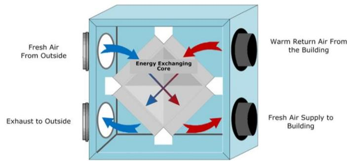
Figure 8.1 Example of Energy Recovery Ventilator
