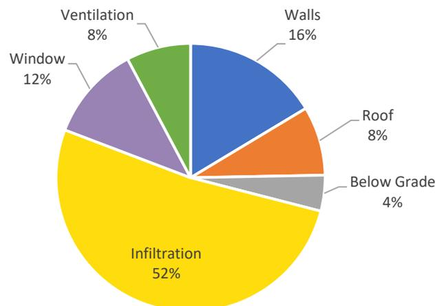
*Figure 6.2 - Enclosure Heat Loss Breakdown*
